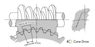
Total load is distributed among more teeth and surface area, greatly increasing torque, load carrying capacity and shock load resistance. Double-enveloping gearsets are more efficient and in a torque-for-torque comparison, are smaller and lighter than standard cylindrical gearsets.
