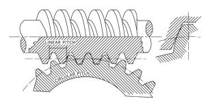
Total load is concentrated to only one-or-two teeth, decreasing torque, load carrying capacity and shock load resistance. As a result, it requires larger, heavier gearsets to produce comparable torque capacity.
