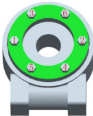
Figure 4. Bolt Torque Sequence
