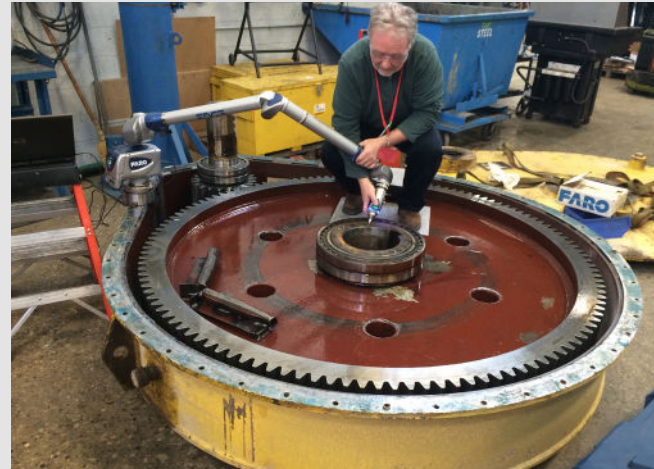
Our FARO arm is state-of-the-art in reverse engineering and inspection technology.
