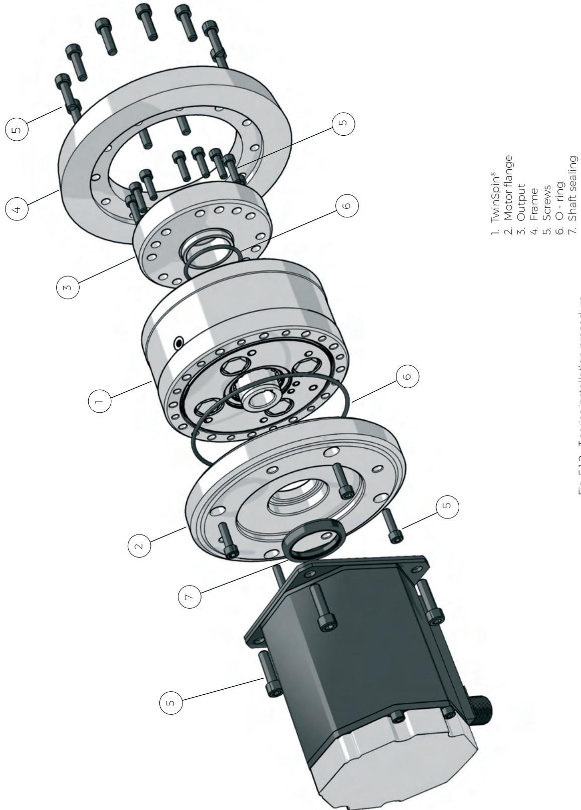
Fig. 5.1.2: T series installation procedure
