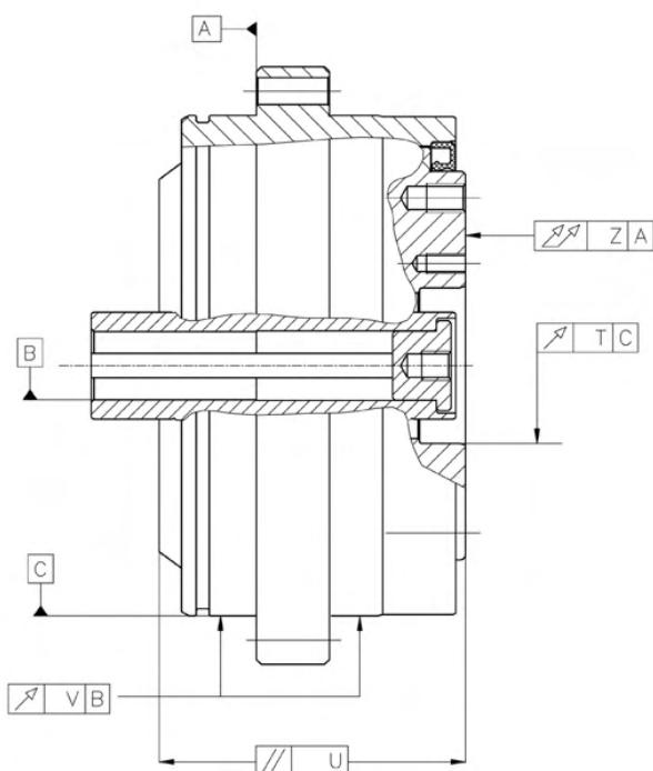
Fig. 5.2.4b: Tolerances of circumferential and face runout in case of direct connection of TwinSpin® high precision reduction gears with servomotor according to DIN 42955 R
