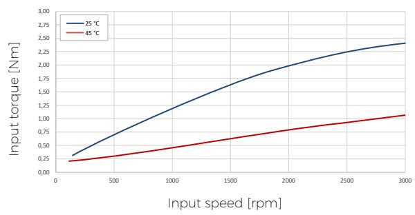
Fig. 3.16: No-load running torque charts
