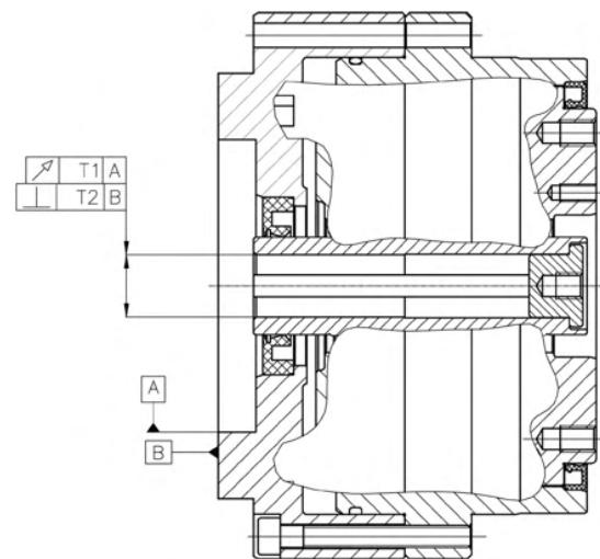
Fig. 5.2.4a: Geometric deviations for connection of the E series TwinSpin® high precision reduction gear flange or of the TwinSpin® E series reduction gear with a motor
