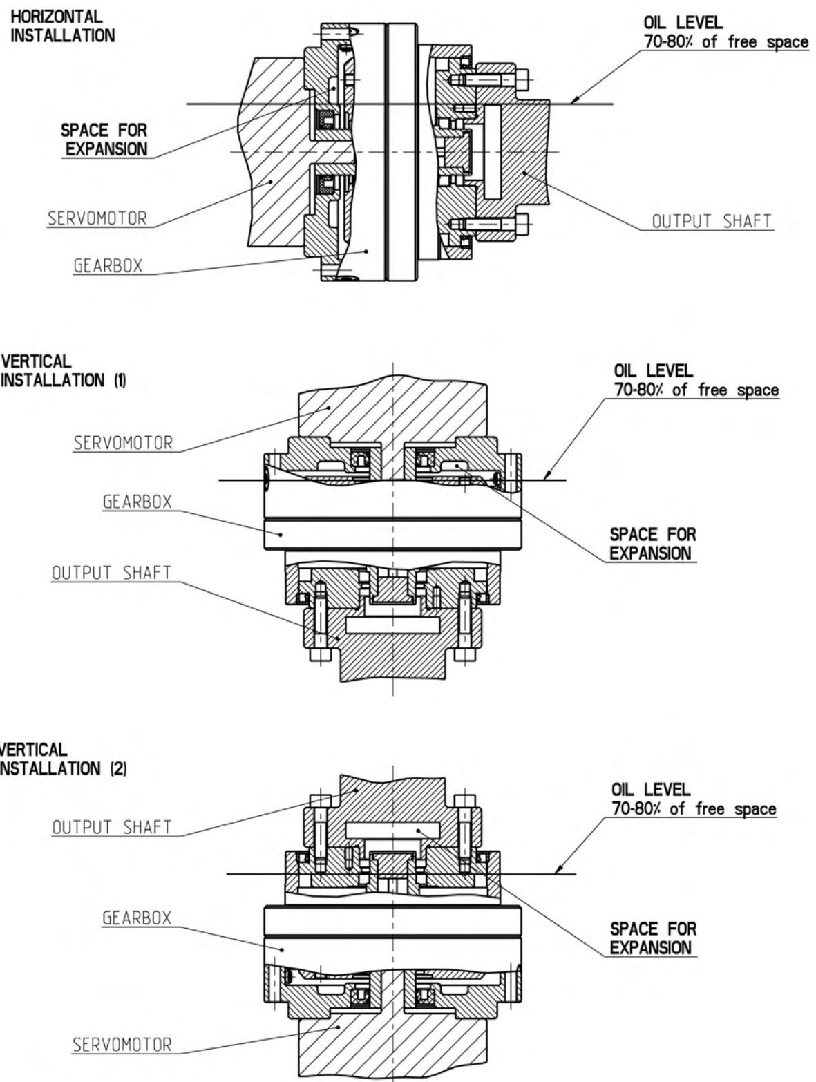
Fig. 5.5a: Lubricant levels in horizontal and vertical positions
