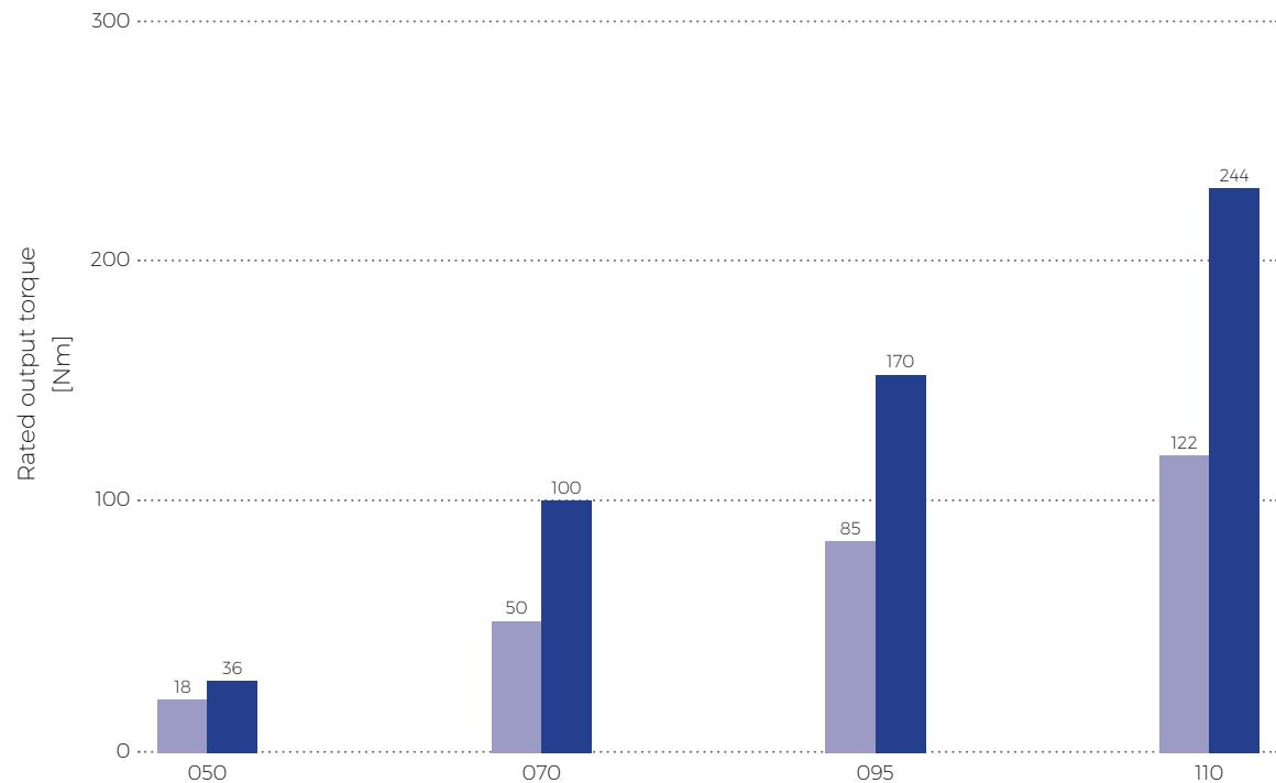
Tab. 8.3a: Rated output torque
