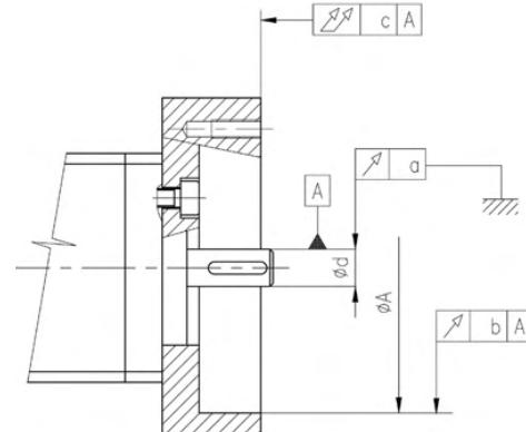
Fig. 5.4.3: Tolerances of M series connecting parts
