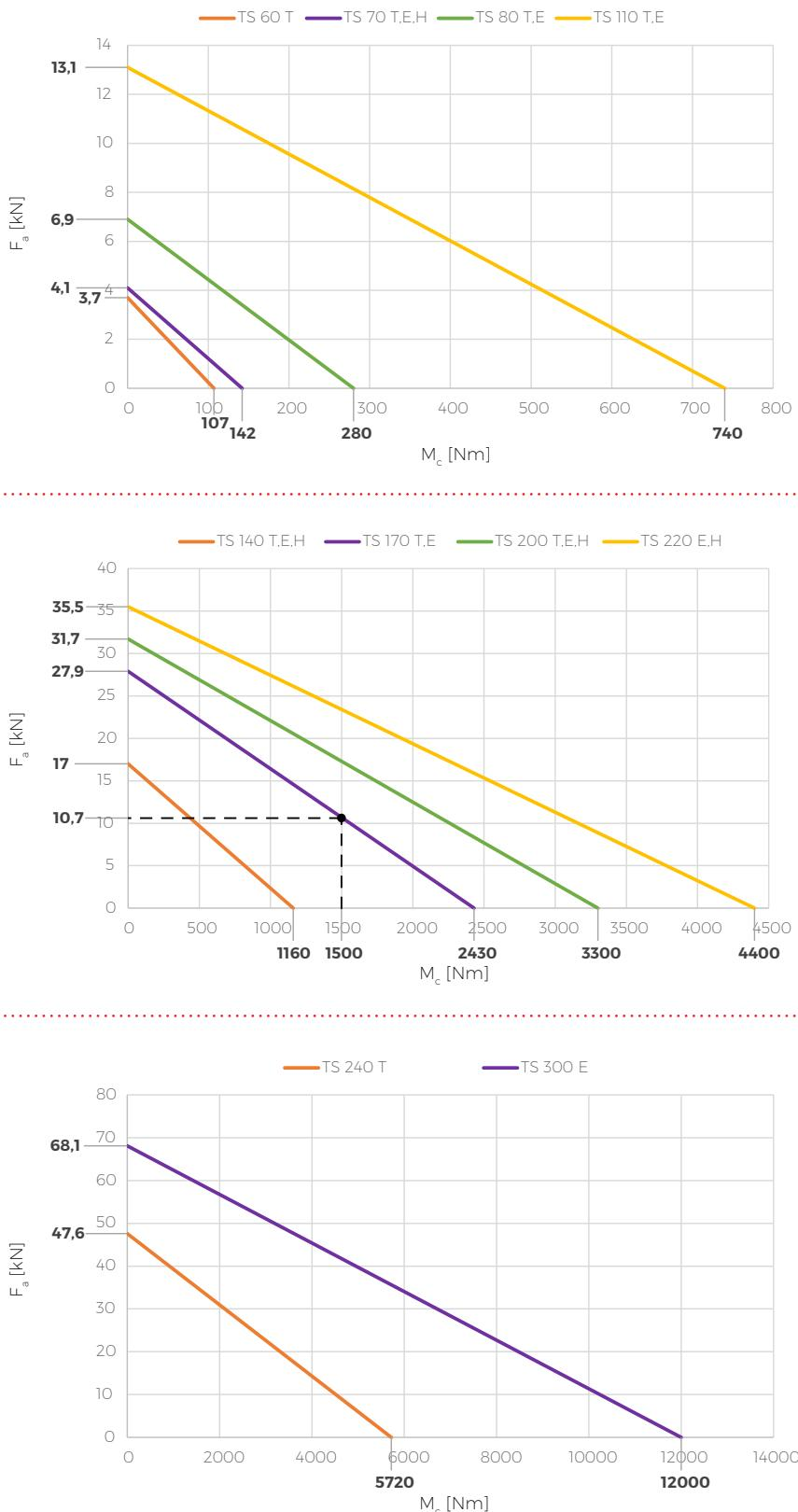
Fig. 3.5: Relation between the moment and axial force
