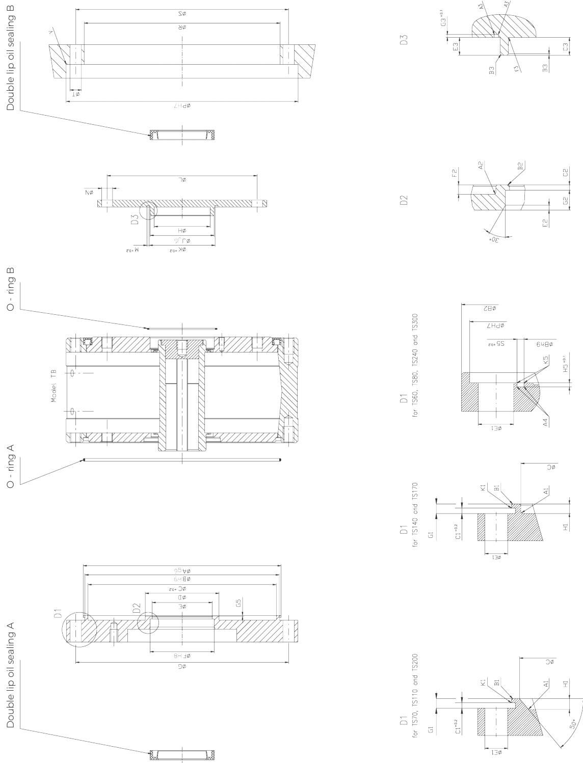
Fig. 5.1.4: Dimensions of the TwinSpin® T series reduction gear input and output flanges
