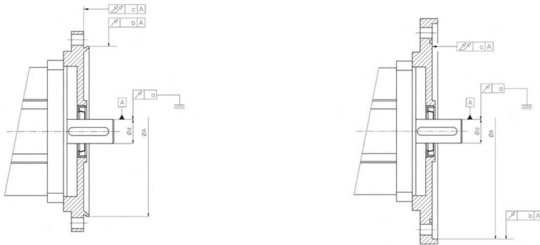
Fig. 5.1.5: Required tolerances of the T series
