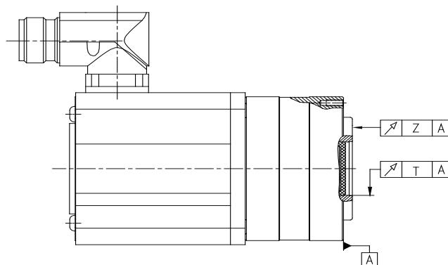
Fig. 8.9.a: Axial and radial runout to base A
