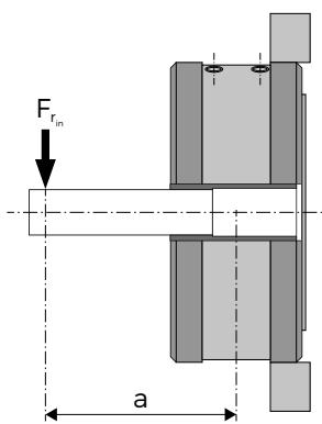
Fig. 3.12a: Radial load of the T, E, H series input shaft
