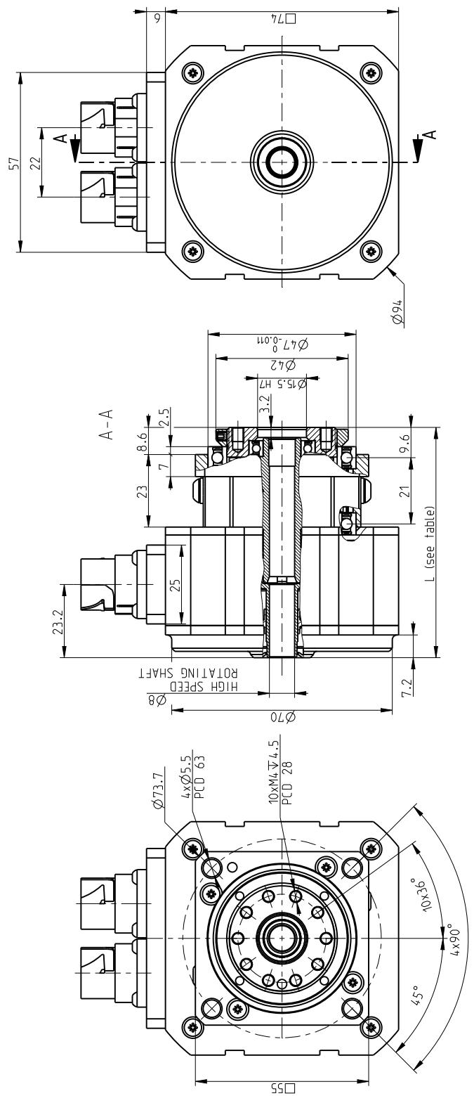
Hollow shaft rotates at motor speed
