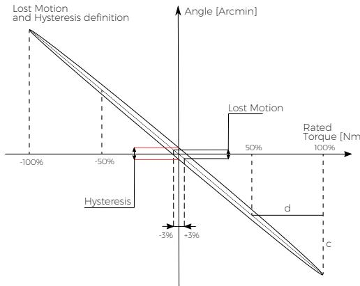
Fig. 3.7a: Hysteresis curve and the definition of stiffness
